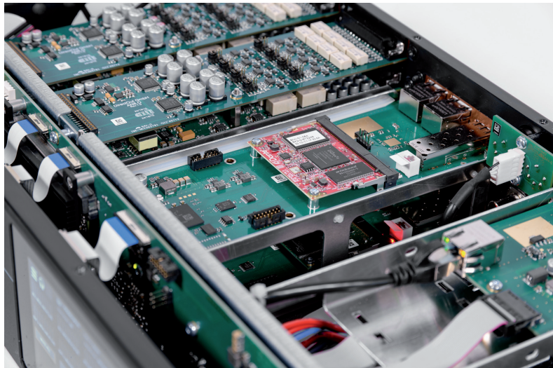
Dante IO card with the Brooklyn II module in the front of the picture, behind it two analogue IOs with optional AN8.0 output board
